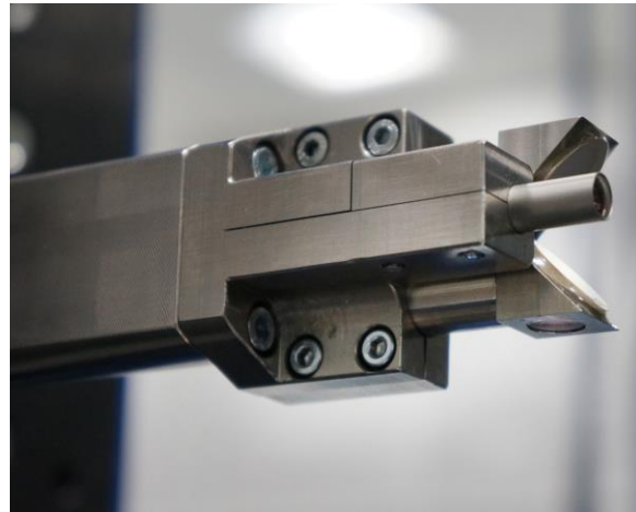
Sensor for the measurement of the outer cell diameter
