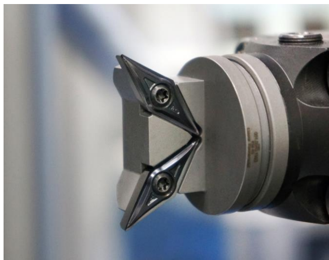
Tool wear has to be controlled before finishing cut
