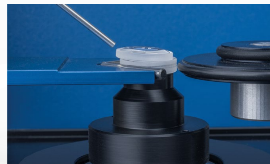
Lens alignment with LensAlign 2D Air on a lens rotation device
